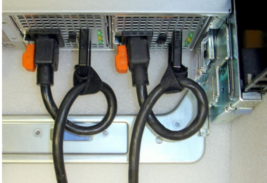
Figure 2: Routing Power Cables Through the Strain Reliefs
